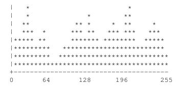
The histogram below corresponds to an image of a white object with a black background. In this case the histogram would be useful in choosing a threshold to use to turn the image into a real black and white image. (BTW, you would choose the threshold to be at about 150).
